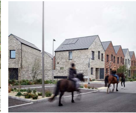
St Chads Development, Essex Shared surface 'home zones' are designed to prioritise pedestrians and cyclists, while reducing vehicular speed.
